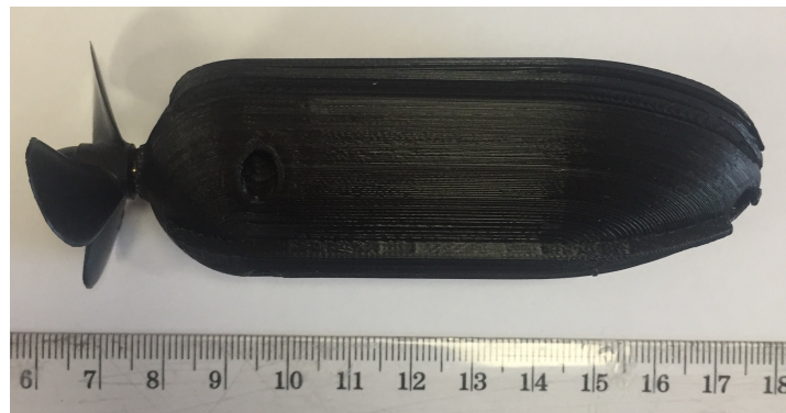
Figure 2. Custom built autonomous submersible robot.
